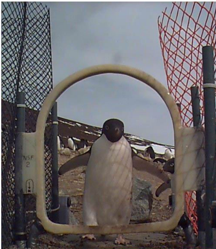
Hoop-coil weighbridge optimizes RFID reading by respecting physics and penguin behaviour Source: Beigel Technology Corp
